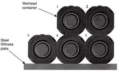
Arrangement of Test Assemblies (End View)
