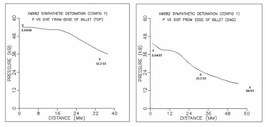
Figure #7 (U) Adjacent and diagonal pressure time histories (line GD-OTS, x – ARDEC)
