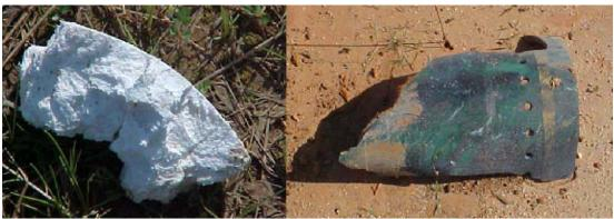
Figure #3 (U) Test #1 unreacted PBXN-9 and large warhead case fragment
