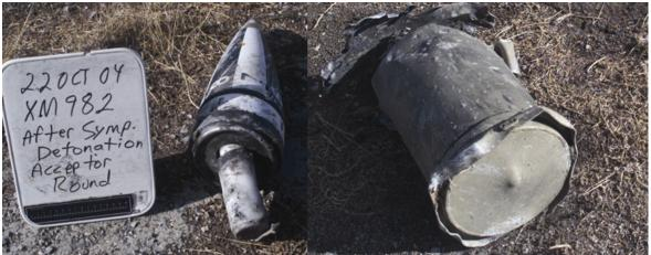
Figure #12 (U) Recovered nose w/FSA and acceptor shipping container (front)
